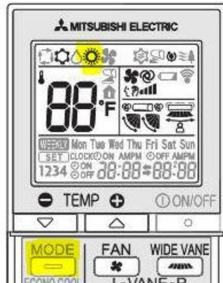
Set the CERV 2° higher than the heat pump – this allows the CERV to act as the primary heat source. If you want to change the temperature, adjust both the heat pump and CERV to maintain the 2° spread. Set the CERV cooling set point at 90° to prevent any cooling from occurring.
